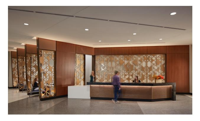
(Oakland, CA) May 2020 - Móz Designs recently completed the striking metal elements at Texas Health Resources designed by HKS Dallas. Móz fabricated 80 metal panels for the project totaling 2,000 square feet of 3/16" aluminum in their Laser Cut Deco pattern in Classic Light Champagne with a Fog grain and polycoat matte finish.
