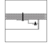
Detail showing an End Key Bar attached to plywood with one outer finished end panel attached.
