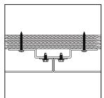
Detail showing a Mid Key Bar attached to plywood with two typical mid panels attached.
