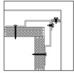
Detail showing a Corner Key Bar attached to plywood with two end corner panels attached.
