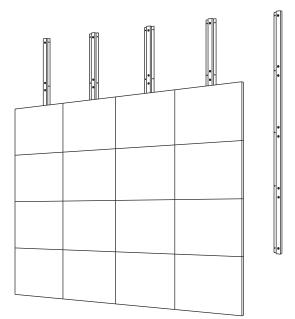
Layout A. Square Installation This example uses 16, 24x 36" panels, with 2 End Key Bars and 3 Mid Key Bars.
