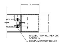
Installation notes: Fasteners and mounting substrate to be provided by others. Install on a straight, flat surface for best performance and alignment.
